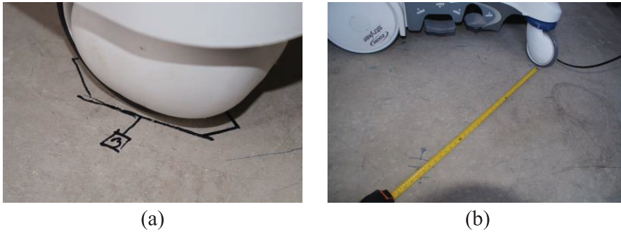
Figure 10. Wheel's initial and final position and orientation of: (a) patient bed PB2, and (b) stretcher PS1 during the seismic tests.
