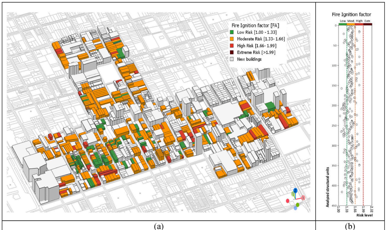
Fig. 8. (A) Mapping and (b) results of fire ignition analysis of Yungay typical zone.
