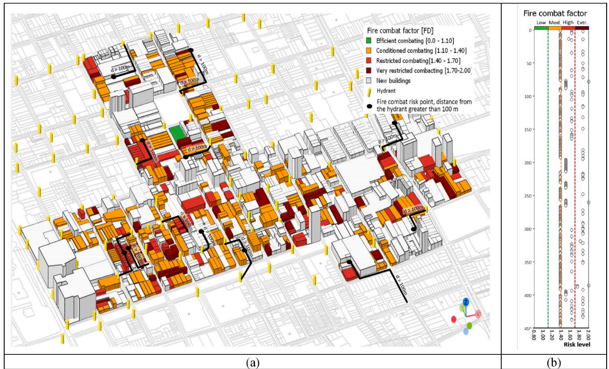
Fig. 11. Fire combat results: (a) Mapping and (b) classification of buildings.
