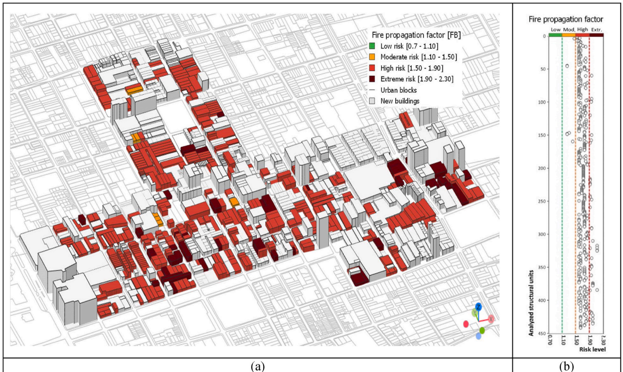
Fig. 9. (A) Mapping and (b) results of fire propagation analysis of Yungay typical zone.
